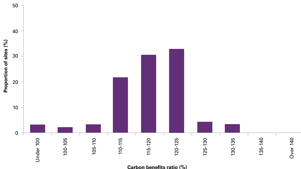
Figure 3.13 Small commercial micro-CHP carbon benefits ratio distribution (monthly data)
